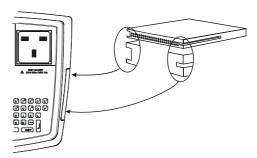
Figure 3. Inserting the CF card
