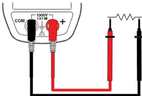
An audible signal is emitted if there is continuity, and the measured value is displayed on the screen.
