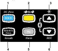
Figure 3: the keys of the keypad
