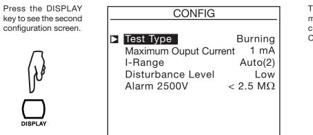
The  $\blacktriangle \nabla$  keys are used to select the measurement configuration. The chosen configuration is validated by pressing the CONFIG key again.
