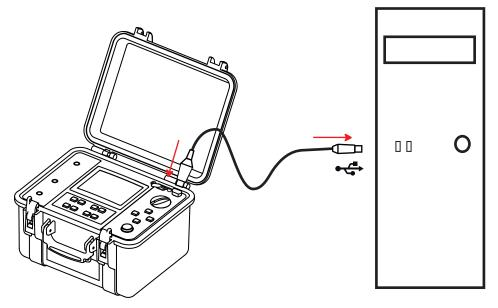
When in communication with a PC, the instrument displays REMOTE and no longer reacts to the user's commands. The keys and the rotary switch are inactive, except for stopping the instrument (OFF setting). To use the data transfer software, refer to the on-line help.
