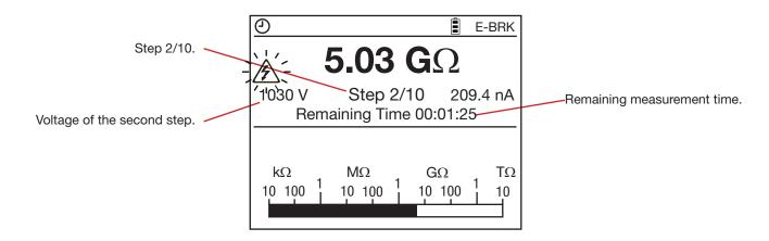
You can view the resistance, voltage, and current vs. time curves by pressing the GRAPH key. For more details, refer to § 4.5.
