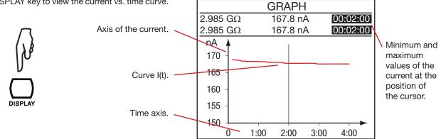
The  $\blacktriangleleft$  keys are used to move along the curve to display the exact values of each sample. It is possible to zoom, as in the case of the R(t) and U(t) curves.
