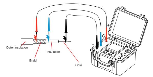
Using the guard eliminates the influence of the surface leakage current.
