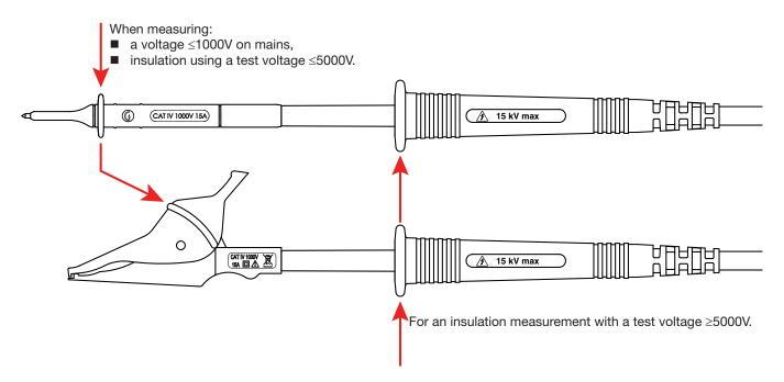
Measurements of voltages  $\geq$ 1000V on mains must be made using the test probes only, with the user's hands behind the guard on the lead.
