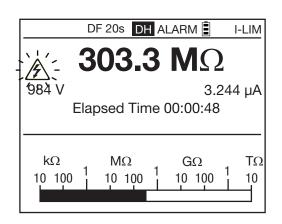
Selecting digital filtering (DF) is recommended for measurements of fluctuating high insulation resistance values. Such fluctuations may be due to hand effects, fluctuating capacitances in the device tested, insulation that varies because of conducting dust, an ionizing and polarizing effect of this dust, etc., or again to the presence of an AC voltage superposed on the measurement.
