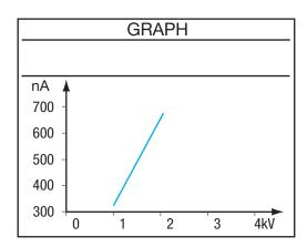
This curve is useful primarily in the case of a measurement in U-RAMP mode. There is no cursor and it is not possible to zoom on this curve.
