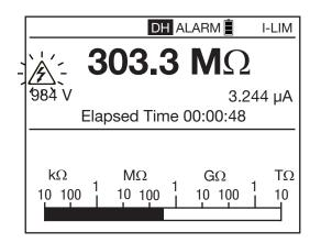
Complementing this, the FILTER key can be used to activate and deactivate a digital filter for the insulation measurements. This filter affects only the display (which is smoothed), not the measurements. The recorded data therefore remain raw (no filter).
