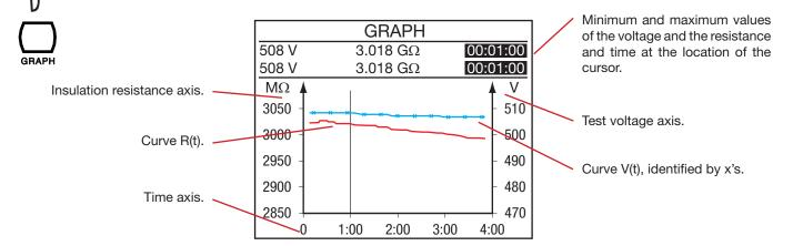
This curve is plotted using samples recorded during the measurement.
