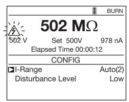
Use the  $\blacktriangleleft \triangleright$  and  $\blacktriangle \nabla$  keys to modify the measurement current range:
