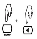
Press the TEMP key, then the < key, to return to the list of recorded measurements..
