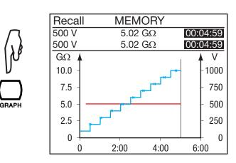
Press the GRAPH key to exit from the curve. In the case of a U-FIXED or U-VAR. measurement, you can press the TEMP key to view the information concerning the temperature.
