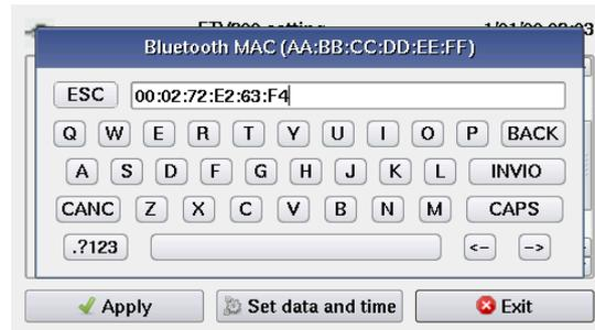
**NOTE:** For the Bluetooth devices of the instrument and the remote unit to be able to communicate, the MAC number of the Bluetooth adapter used on the instrument must be set in the Bluetooth device used on the remote unit.
