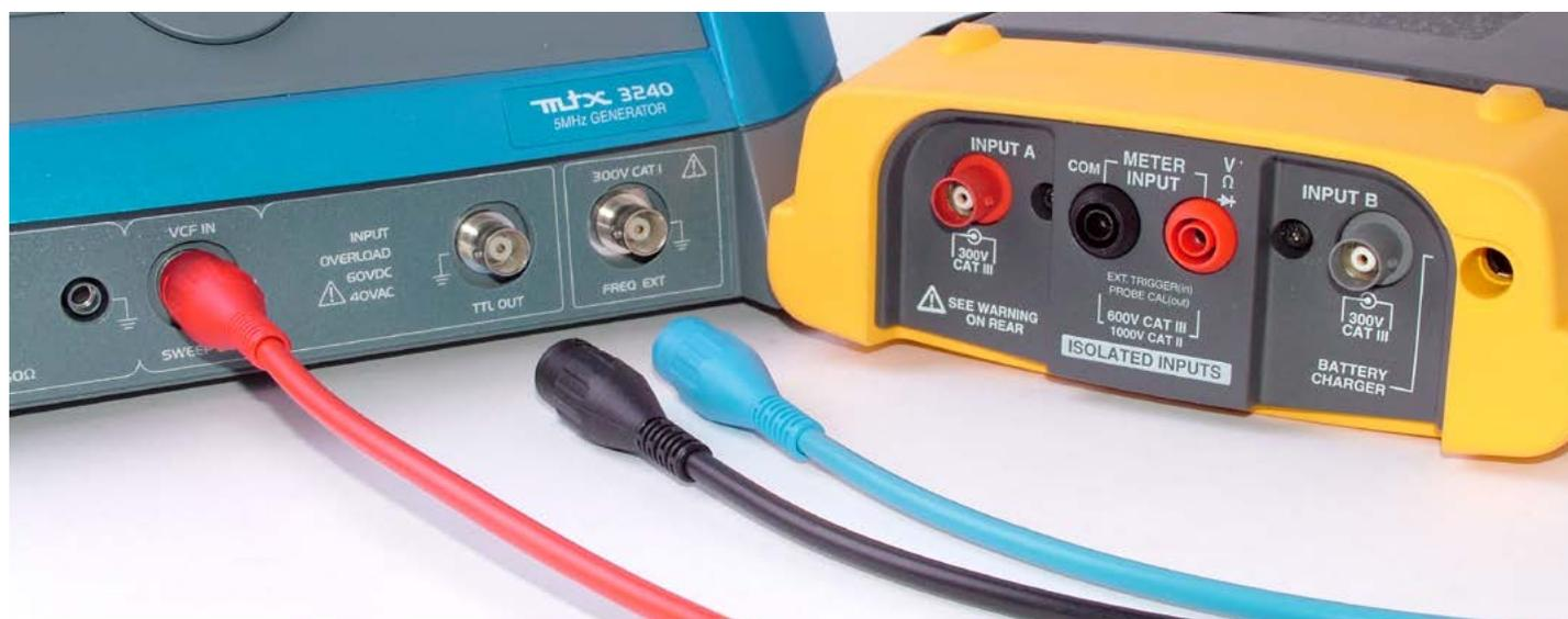
Test leads with touch-protected BNC plugs can be connected to devices with insulated and conventional BNC sockets.
