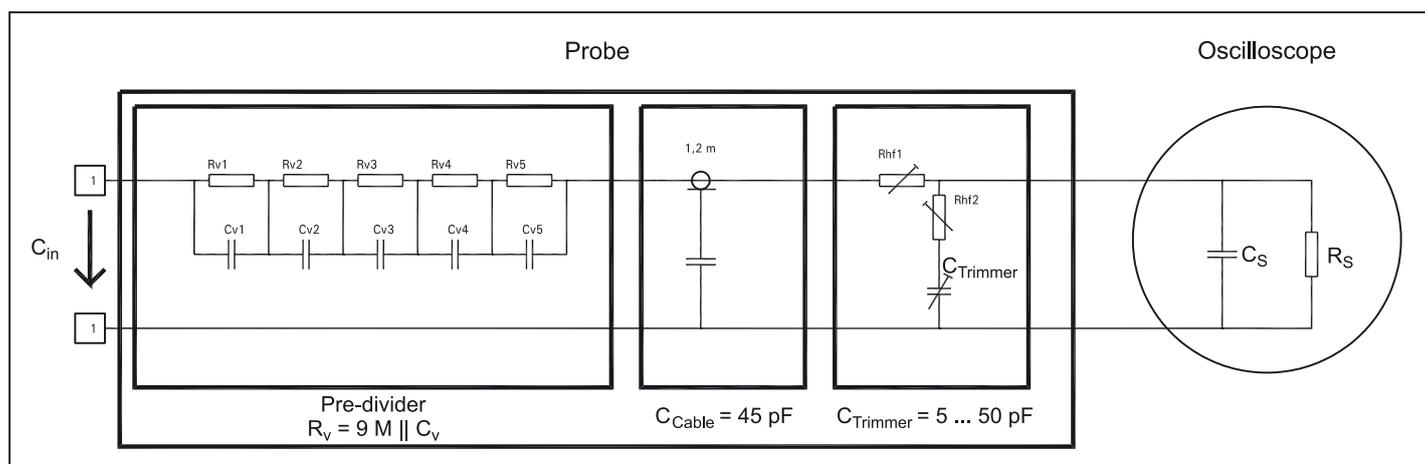
Schematic diagram of a passive 10:1 test probe
