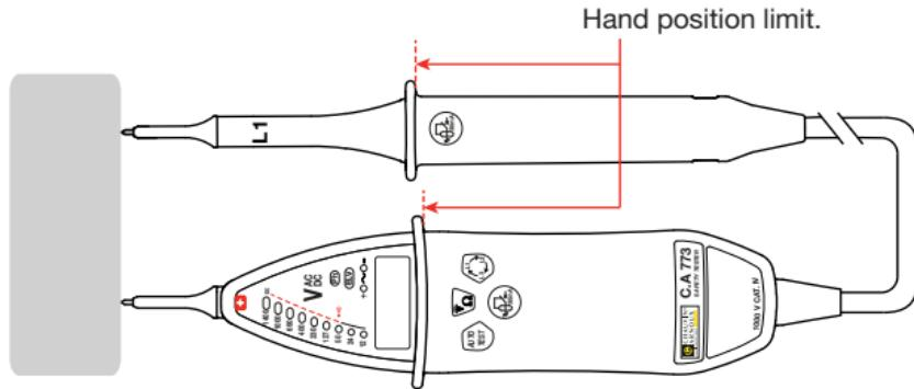
Place the test probes on the element to be tested, and hold them firmly in contact.
