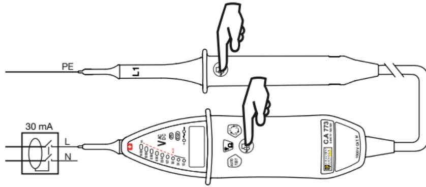
If the voltage measured is between 8 Vrms and 400 Vrms, the test is triggered.
