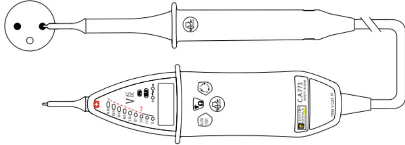
If the test probe is on the phase, the **Ph** (phase) indicator flashes and the device beeps.
