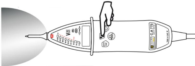
To switch the light off, press the **Ω** button again, or wait for it to extinguish itself automatically after about 10 seconds.
