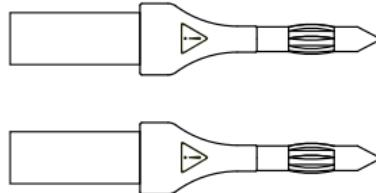
Red IP2X test probe Ø 2 mm (one red and one black)..... P01102127Z
