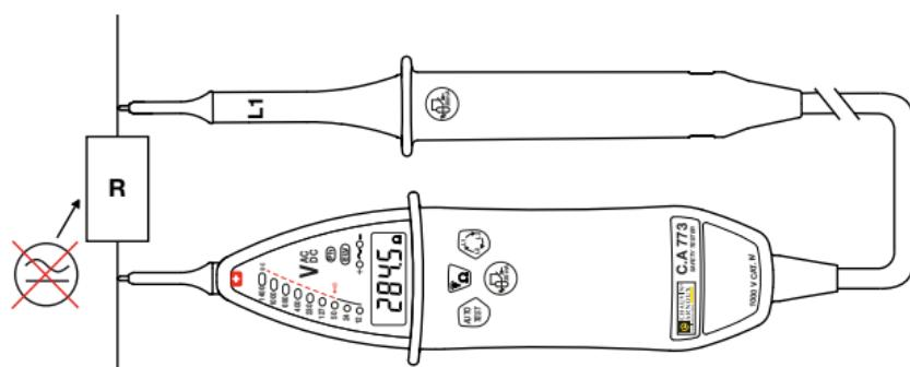
If the device has been idle for more than 10 minutes or if it was set to stand-by mode, run a self-test first, to place it in active stand-by.
