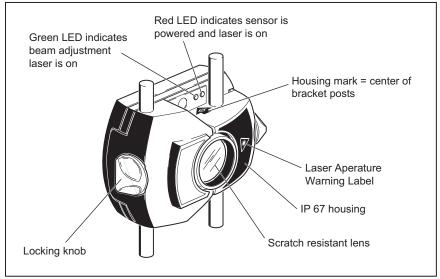
Figure 4-4. Parts of sensor
