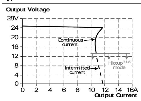
Fig. 5-2 Short-circuit on output, Hiccup<sup>PLUS</sup> mode, typ.
