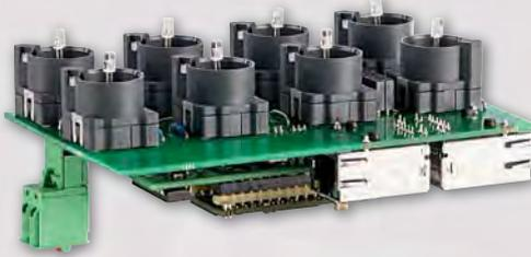
ProfiNET I/O specification: 2 ports with transformer
