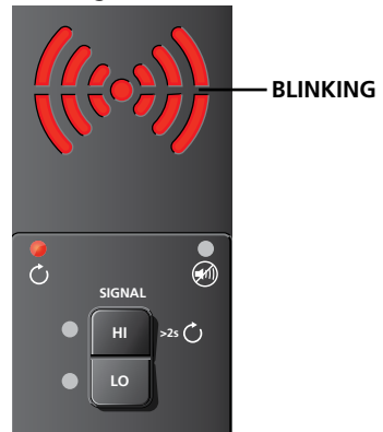
Figure 4.12b: Transmitter screen showing signal in LOOP mode
