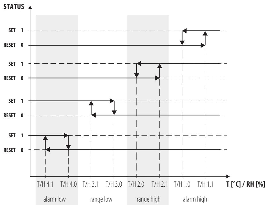
The bit "Alarm high" is set if T/H1.1 is reached / exceeded ( $\geq$ ). It is reset if T/H1.0 is reached / undershot ( $\leq$ ).
