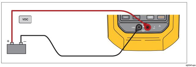
Figure 17. VDC Measurement Connections
