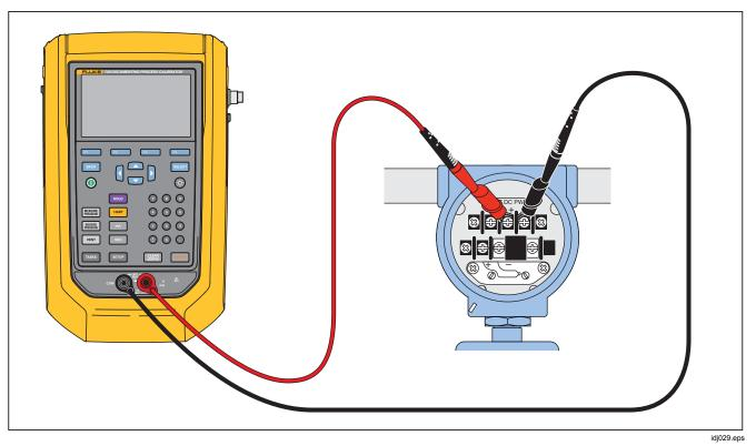
Figure 16. Connection with Loop Power Enabled
