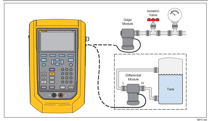
Figure 19. Pressure Module Connections
