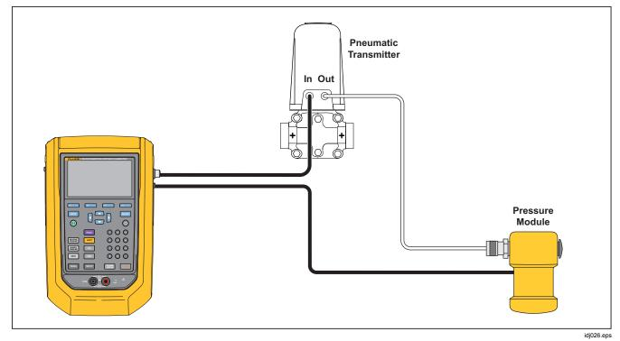
Figure 15. Pressure Transmitter (P/P) Connections
