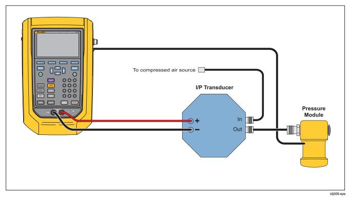
Figure 13. Current to Pressure Test (I/P) with External Pressure Module
