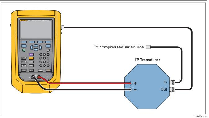
Figure 14. Current to Pressure Test (I/P) with Internal Connections
