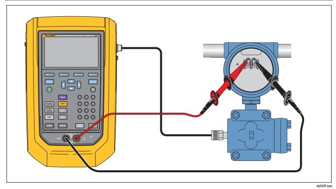
Figure 11. Pressure Transmitter (P/I) Task Connections
