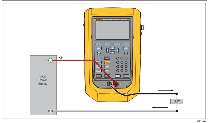
Figure 21. Connections to Simulate a 4 to 20 mA Transmitter
