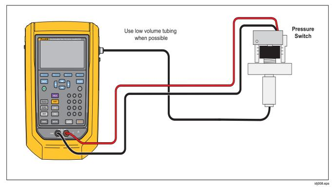
Figure 12. Switch Test Connections
