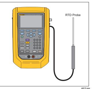
Figure 20. Temperature Probe Connection
