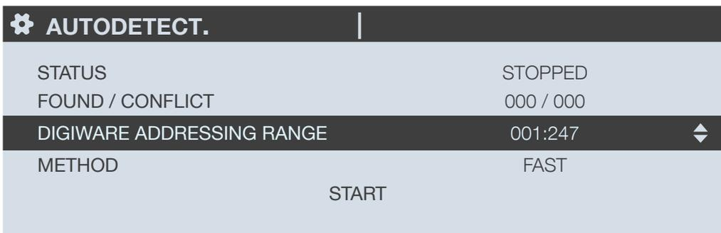
This allows you to allocate Modbus addresses to the connected devices within a specific range:
