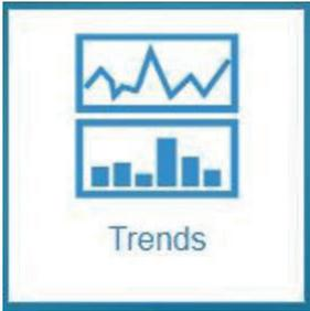
The **Trends** menu displays measurement logs (historical measurements) collected by the devices over the time period selected in the left pane.
