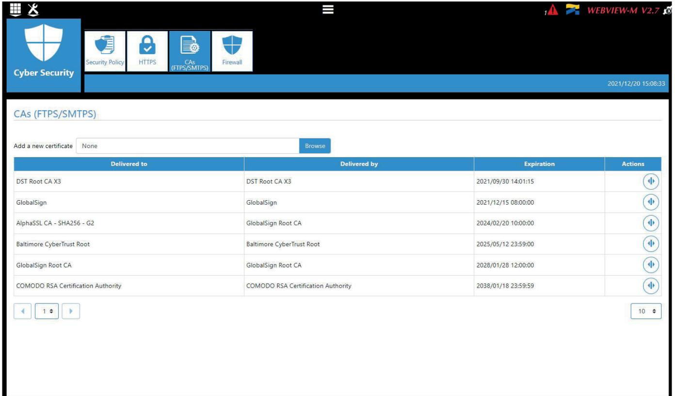
The screenshot shows the 'CAs (FTPS/SMTSPS)' tab in the Cyber Security interface. At the top, there is a navigation bar with icons for Security Policy, HTTPS, CAs (FTPS/SMTSPS), and Firewall. Below the navigation bar, there is a section for adding a new certificate, with a dropdown menu set to 'None' and a 'Browse' button. The main content area displays a table of installed Certificate Authorities.
