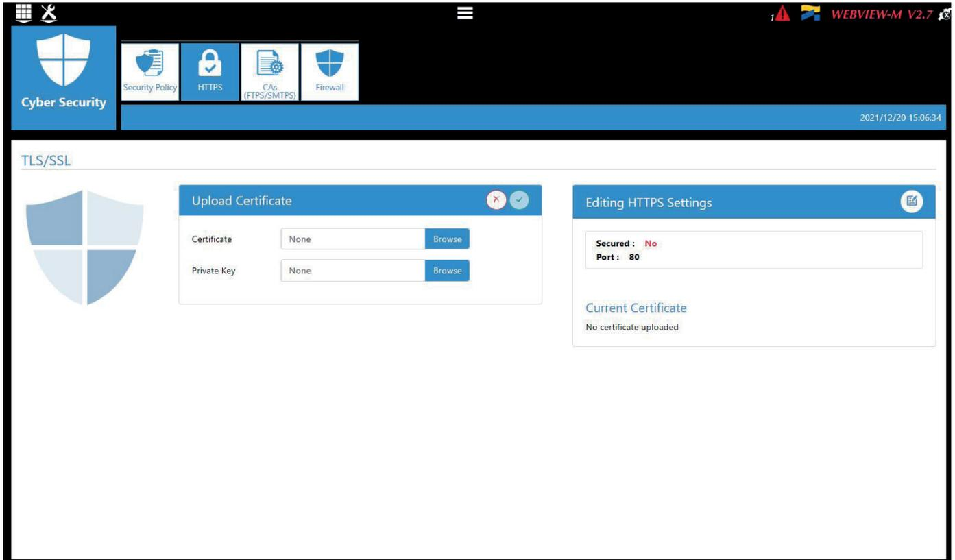
The M-xx gateway / D-xx display will accept a digital certificate under the .pem format. Once a digital certificate and private key has been uploaded, you can edit HTTPS settings to secure the web navigation.
