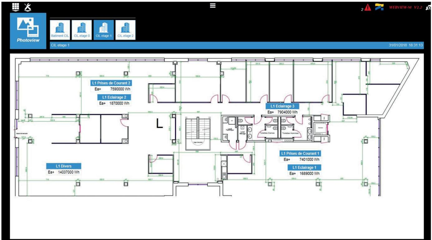
When clicking on the various added elements (e.g. a measurement table), the user is redirected to the “Monitor” menu of the associated device.
