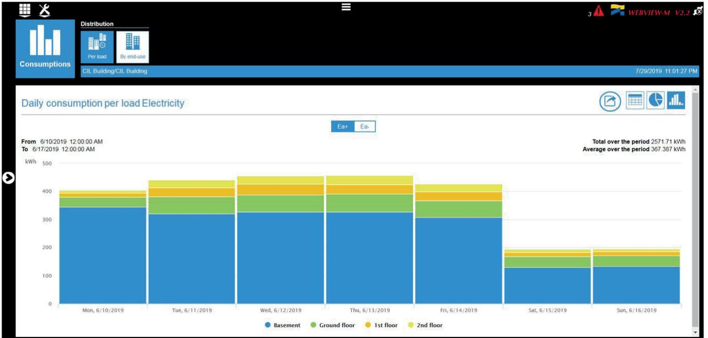
By clicking on one of the load names ("Basement" in the example below), it can be removed from the graph. The total consumption value given in the top right corner is also updated when loads are selected / unselected:
