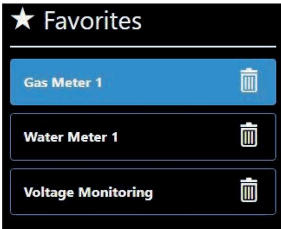
Only available under the “Trends” menu, the Favourites allows you to save your frequently consulted measurement logs. (For example, the electrical parameters of a process or load curve correlated with one or several influence factors).
