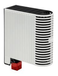
Compact loop heater based on PTC heating elements for heating casings with electrical or electronic components. The heater can be used to prevent both low temperatures and condensation on built-in components. Fast electrical contacting through pressure clamps.
