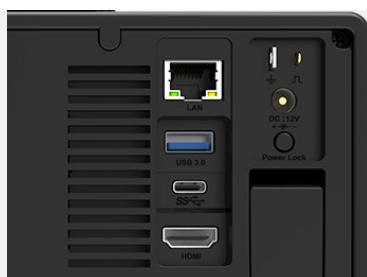
► Standard USB 3.0 Host, Type-C, LAN, HDMI, calibration square wave output interface, Trigger out meet diverse connection needs, enhancing flexibility and convenience of test work. It also supports power lock for safer carrying.
